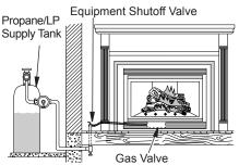
Figure 41 - Checking Gas Joints for Propane/LP Gas Fireplace
